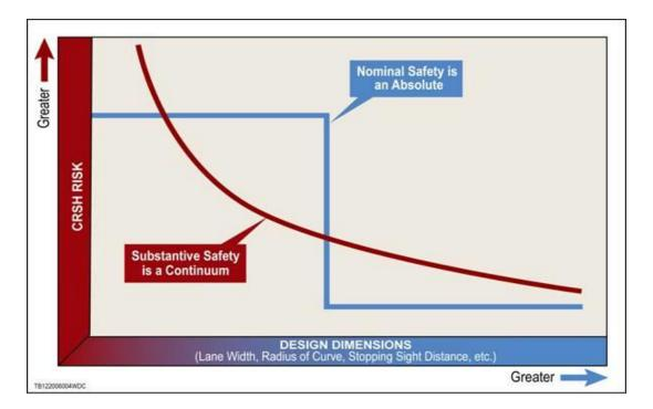
As design manuals are examined, AASHTO's Policy on Geometric Design of Highways and Streets would be considered to contain nominal safety characteristics. In contrast, AASHTO's Highway Safety Manual would be considered to contain substantive safety characteristics.
